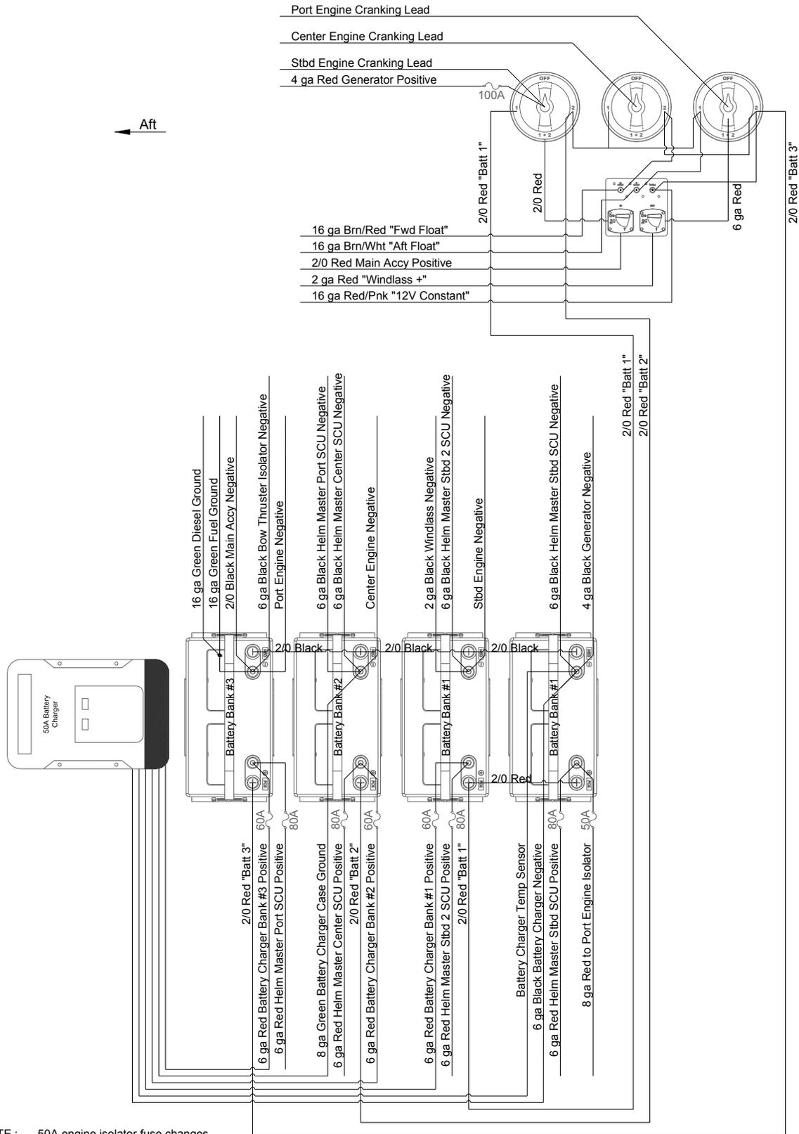
NOTE : 50A engine isolator fuse changes to 100A MRCB if the boat is equipped with V6 engines.
